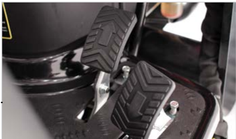
Switch seamlessly between forward and reverse with two side-by-side hydrostatic transmission pedals.
